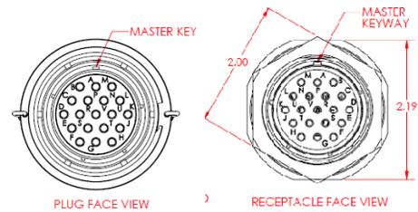
Figure 5. Plug and Receptacle Face Patterns: 19 way Base
