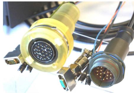
Figure 6. Plug and Receptacle Shown Together
